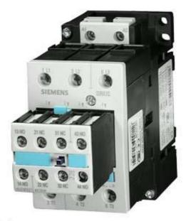
Power contactor, AC-3 32 A, 15 kW / 400 V 400 V AC, 50 Hz / 60 Hz, 440 V, 60 Hz, 2 NO + 2 NC, 3-pole, Size S2, Screw terminal !!! Phased-out product !!! Successor is SIRIUS 3RT2 Preferred successor type is
