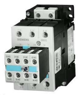
Power contactor, AC-3 40 A, 18.5 kW / 400 V 400 V AC, 50 Hz / 60 Hz, 440 V, 60 Hz, 2 NO + 2 NC, 3-pole, Size S2, Screw terminal !!! Phased-out product !!! Successor is SIRIUS 3RT2 Preferred successor type is
