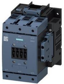
Power contactor, AC-3 115 A, 55 kW / 400 V AC (50-60 Hz) / DC operation 21-27.3 V UC Auxiliary contacts 2 NO + 2 NC 3-pole, Size S6 with box terminals Drive: electronic with PLC interface 24 V DC screw terminal
