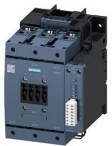
Power contactor, AC-3 115 A, 55 kW / 400 V AC (50-60 Hz) / DC operation 96-127 V UC Auxiliary contacts 1 NO + 1 NC 3-pole, Size S6 with box terminals Drive: electronic with PLC / SIMOCODE interface and RLT signal
