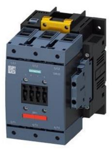
Power contactor, AC-3 115 A, 55 kW / 400 V Coil AC 50/60 Hz and DC 96-127 V x (0.8-1.1) F-PLC input 24 V DC 3-pole size S6 Auxiliary contacts 2 NO + 2 NC cannot be dissolved (SUVA) Main circuit: Box terminal Control and auxiliary circuit: screw terminal
