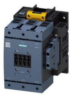
Power contactor, AC-3 115 A, 55 kW / 400 V Coil AC 50/60 Hz and DC 96-127 V x (0.8-1.1) F-PLC input 24 V DC 3-pole size S6 Auxiliary contacts 2 NO + 2 NC Main circuit: Box terminal Control and auxiliary circuit: screw terminal
