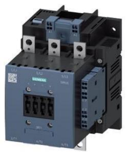
Power contactor, AC-3 115 A, 55 kW / 400 V AC (50-60 Hz) / DC operation 21-27 UC, 3 V Auxiliary contacts 2 NO + 2 NC 3-pole, Size S6 Busbar connections Drive: electronic with PLC interface 24 V DC Spring-type terminal
