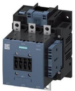
Power contactor, AC-3 115 A, 55 kW / 400 V AC (50-60 Hz) / DC operation 96-127 V UC Auxiliary contacts 2 NO + 2 NC 3-pole, Size S6 Busbar connections Drive: electronic with PLC interface 24 V DC Spring-type terminal
