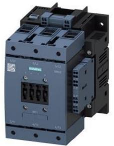
Power contactor, AC-3 115 A, 55 kW / 400 V AC (50-60 Hz) / DC operation 21-27 UC, 3 V Auxiliary contacts 2 NO + 2 NC 3-pole, Size S6 with box terminals Drive: electronic with PLC interface 24 V DC Spring-type terminal
