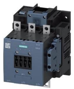
Power contactor, AC-3 115 A, 55 kW / 400 V AC (50-60 Hz) / DC operation 96-127 V UC Auxiliary contacts 2 NO + 2 NC 3-pole, Size S6 Busbar connections Drive: electronic with PLC interface 24 V DC screw terminal
