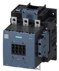
Power contactor, AC-3 115 A, 55 kW / 400 V AC (50-60 Hz) / DC operation 200-277 V UC Auxiliary contacts 2 NO + 2 NC 3-pole, Size S6 Busbar connections Drive: electronic with PLC interface 24 V DC screw terminal
