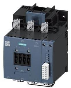
Power contactor, AC-3 115 A, 55 kW / 400 V AC (50-60 Hz) / DC operation 200-277 V UC Auxiliary contacts 1 NO + 1 NC 3-pole, Size S6 Busbar connections Drive: electronic with PLC / SIMOCODE interface and RLT signal
