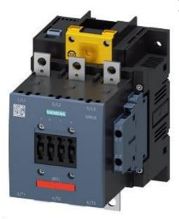
Power contactor, AC-3 115 A, 55 kW / 400 V Coil AC 50/60 Hz and DC 96-127 V x (0.8-1.1) F-PLC input 24 V DC 3-pole size S6 Auxiliary contacts 2 NO + 2 NC cannot be dissolved (SUVA) Main circuit: Busbar Control and auxiliary circuit: screw terminal
