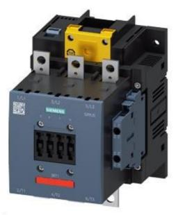
Power contactor, AC-3 115 A, 55 kW / 400 V Coil AC 50/60 Hz and DC 200-277 V x (0.8-1.1) F-PLC input 24 V DC 3-pole size S6 Auxiliary contacts 2 NO + 2 NC cannot be dissolved (SUVA) Main circuit: Busbar Control and auxiliary circuit: screw terminal
