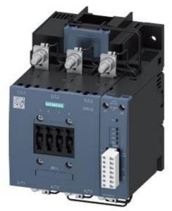
Power contactor, AC-3 150 A, 75 kW / 400 V AC (50-60 Hz) / DC operation 96-127 V UC Auxiliary contacts 1 NO + 1 NC 3-pole, Size S6 Busbar connections Drive: electronic with PLC / SIMOCODE interface and RLT signal
