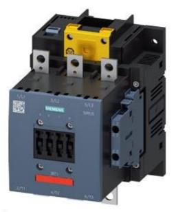
Power contactor, AC-3 150 A, 75 kW / 400 V Coil AC 50/60 Hz and DC 96-127 V x (0.8-1.1) F-PLC input 24 V DC 3-pole size S6 Auxiliary contacts 2 NO + 2 NC cannot be dissolved (SUVA) Main circuit: Busbar Control and auxiliary circuit: screw terminal
