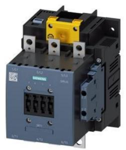
Power contactor, AC-3 150 A, 75 kW / 400 V Coil AC 50/60 Hz and DC 96-127 V x (0.8-1.1) F-PLC input 24 V DC 3-pole size S6 Auxiliary contacts 2 NO + 2 NC Main circuit: Busbar Control and auxiliary circuit: screw terminal
