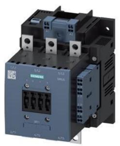
Power contactor, AC-3 185 A, 90 kW / 400 V AC (50-60 Hz) / DC operation 21-27 UC, 3 V Auxiliary contacts 2 NO + 2 NC 3-pole, Size S6 Busbar connections Drive: electronic with PLC interface 24 V DC Spring-type terminal
