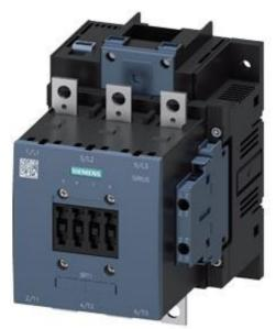
Power contactor, AC-3 185 A, 90 kW / 400 V AC (50-60 Hz) / DC operation 96-127 V UC Auxiliary contacts 2 NO + 2 NC 3-pole, Size S6 Busbar connections Drive: electronic with PLC interface 24 V DC screw terminal
