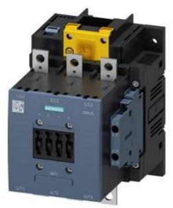
Power contactor, AC-3 185 A, 90 kW / 400 V Coil AC 50/60 Hz and DC 200-277 V x (0.8-1.1) F-PLC input 24 V DC 3-pole size S6 Auxiliary contacts 2 NO + 2 NC Main circuit: Busbar Control and auxiliary circuit: screw terminal
