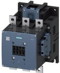
Power contactor, AC-3 225 A, 110 kW / 400 V AC (50-60 Hz) / DC operation 200-277 V UC Auxiliary contacts 2 NO + 2 NC 3-pole, Size S10 Busbar connections Drive: electronic with PLC interface 24 V
