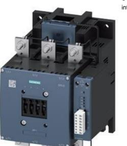
Power contactor, AC-3 225 A, 110 kW / 400 V AC (50-60 Hz) / DC operation 96-127 V UC Auxiliary contacts 1 NO + 1 NC 3-pole, Size S10 Busbar connections Drive: electronic with PLC / SIMOCODE interface and RLT signal
