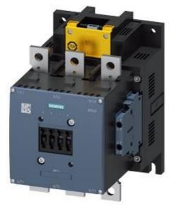
Power contactor, AC-3 225 A, 110 kW / 400 V Coil AC 50/60 Hz and DC 96-127 V x (0.8-1.1) F-PLC input 24 V DC 3-pole size S10 Auxiliary contacts 2 NO + 2 NC Main circuit: Busbar Control and auxiliary circuit: screw terminal
