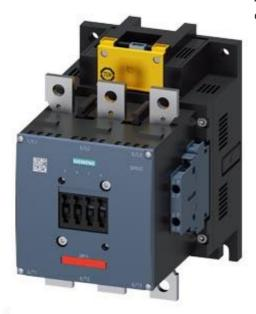
Power contactor, AC-3 225 A, 110 kW / 400 V Coil AC 50/60 Hz and DC 200-277 V x (0.8-1.1) F-PLC input 24 V DC 3-pole size S10 Auxiliary contacts 2 NO + 2 NC cannot be dissolved (SUVA) Main circuit: Busbar Control and auxiliary circuit: screw terminal
