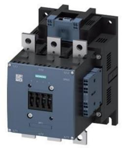
Power contactor, AC-3 265 A, 132 kW / 400 V AC (50-60 Hz) / DC operation 21-27 UC, 3 V Auxiliary contacts 2 NO + 2 NC 3-pole, Size S10 Busbar connections Drive: electronic with PLC interface 24 V DC Spring-type terminal
