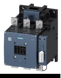
Power contactor, AC-3 265 A, 132 kW / 400 V AC (50-60 Hz) / DC operation 96-127 V UC Auxiliary contacts 1 NO + 1 NC 3-pole, Size S10 Busbar connections Drive: electronic with PLC / SIMOCODE interface and RLT signal
