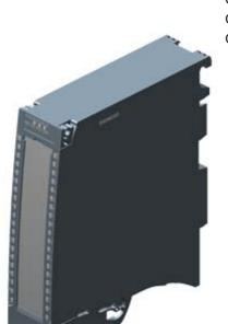
SIPLUS S7-1500 DQ 32x24VDC/0.5A -40 ... +70 DEG C WITH CONFORMAL COATING BasedOn: 6ES7522-1BL01-0AB0 . 32 CHANNELS IN GROUPS OF 8, 4 A PER GROUP; SINGLE-CHANNEL DIAGNOSIS; SUBSTITUTE VALUE
