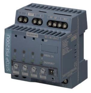
SITOP PSE200U SELECTIVITY MODULE 3A SITOP PSE200U 3 A Selectivity module 4-channel input: DC 24 V/12 A output: 24 V DC/4x 3 A Level adjustable 0.5-3 A mit status message for each output
